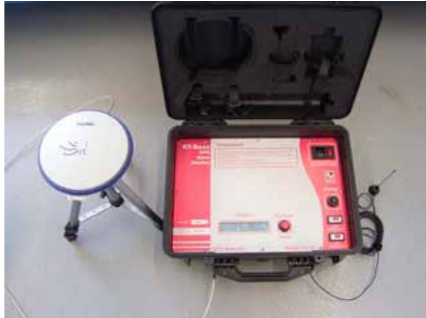
DGPS Base Station
